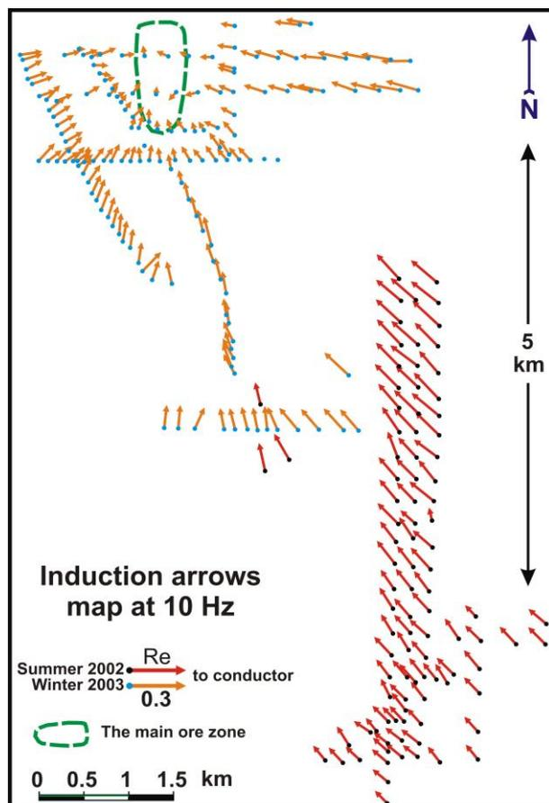
**Figure 4.** Induction arrows map at 10 Hz.
