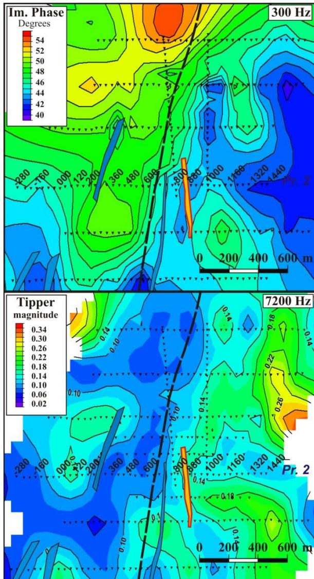
**Figure 3.** Invariant impedance phase map at 300 Hz (a) and Tipper magnitude map at 7200 Hz (b).
