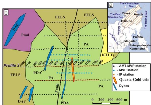
**Figure 1.** Position of Chukotka region on North-East part of Russia (a), geology scheme of investigation area with location of AMT-MVP, MVP and IP stations (b) Legend (b): DAC – Dacite; FELS – 'Felsic' volcanic rocks, undivided - rhyolite, dacitic-rhyolitic lapilli tuff; PDA - Porphyritic dacitic andesite; PA – Porphyritic andesite; PMd – Microdiorite, Porphyritic.
