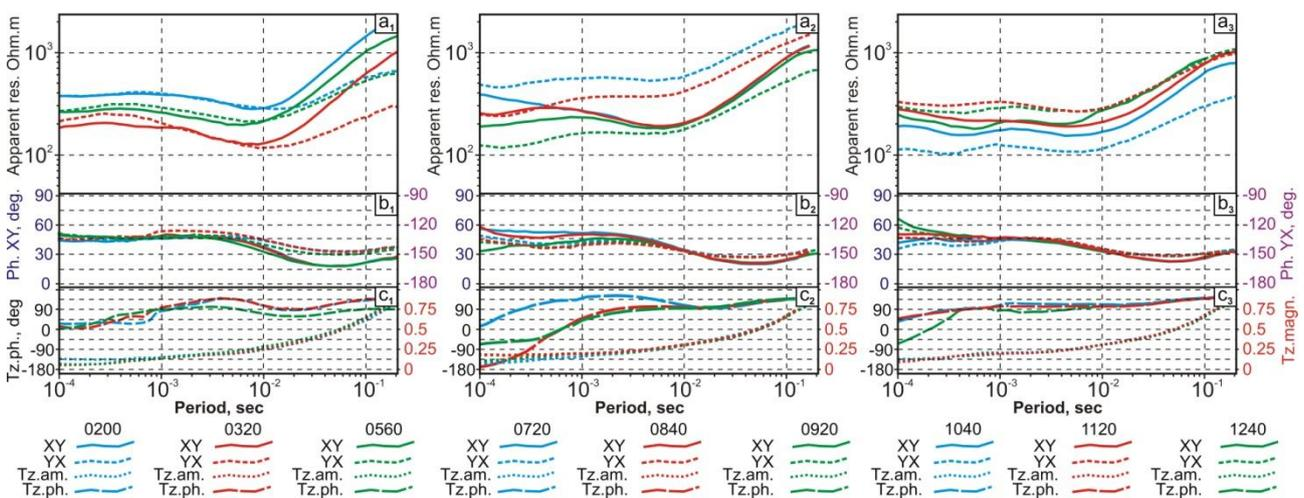
**Figure 2.** Type of AMT-MVP curves for westerly (index 1), nearly (index 2) and easterly (index 3) of vein zone. Type of AMT curves (a, b): apparent resistivity (a) and Impedance phase (b) along XY direction shown by solid line, along YX direction shown by dotted line. MVP curves (c): tipper magnitude shown by dots, tipper phase shown by dotted line. The AMT-MVP station names are shown under the period axes.
